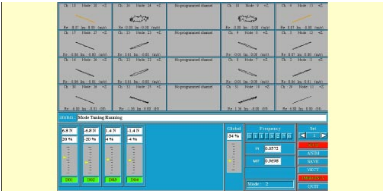
Figure 3. Typical controls and multi-Lissajous display used while tuning a mode. One 'slider' is provided for each shaker and adjusts the relative force (and phase) applied by that driver. A Global slider sets the absolute force levels by varying all drives while maintaining their relative strengths. The exact shaker frequency may be adjusted with 0.1 PPM resolution. Each velocity-versus-force Lissajous figure 'collapses' to a straight line at perfect tuning. Two global indicators aide the iterative tuning: the Phase Indicator (PI) approaches zero while the Modal Indicator Function (MIF) approaches unity as shape-tuning is optimized.
