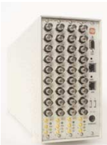
Abacus featuring embedded PC, local disk, up to 32 inputs, eight outputs and eight tacho channels
