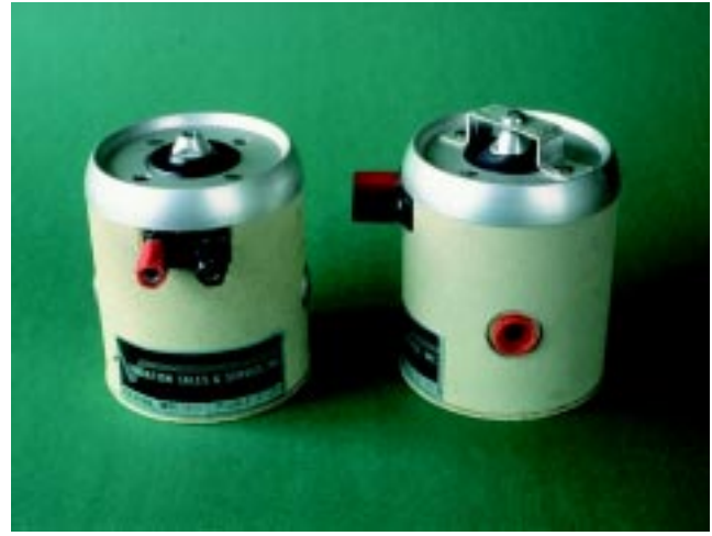
Figure 11. Mechanical configurations for traditional coil impedance tests. The unit on the left is unrestrained, the shaker on the right has its table motion blocked by a bracket.
