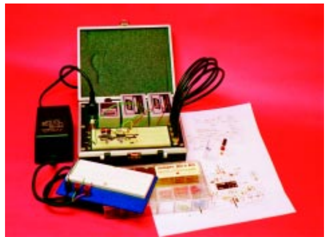
Figure 6. The circuit of Figure 5 was constructed from two integrated circuits (with one amplifier left over!) on a shop-built prototyping rig. The rig contains precision power supplies and a convenient way to interface BNC connectors with the circuit. Commercial development boards, such as that shown, can also be used to build small circuits. Planning the component placement before patching is always a good idea . . . note the pictorial layout.
