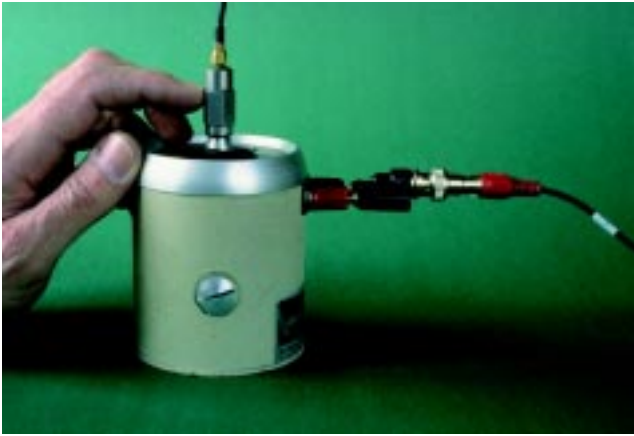
Figure 8. 'Pluck' testing an LDS model V-203 shaker. The finger depresses the table against its limit stop, then releases it abruptly. The voltage generated by the shaker coil is measured with a high impedance instrument. Comparative spectral measurements made between a bare table and one loaded with a known mass permit identifying the suspension parameters.
