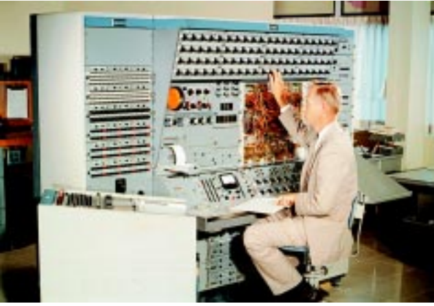
Figure 1. A typical analog computer of circa 1960 featured a removable program patch board, banks of \pm 100 Volt (vacuum tube!) amplifiers and hundreds of coefficient potentiometers plus other support circuits and accessories. The unit shown is an EAI model 231-R, one of five such ‘workhorses’ housed at the GMPG Noise and Vibration Laboratory and frequently driven in tandem! The human workhorse is far more unique; Tom Harris was my boss, mentor and best friend during my tenure with General Motors.
